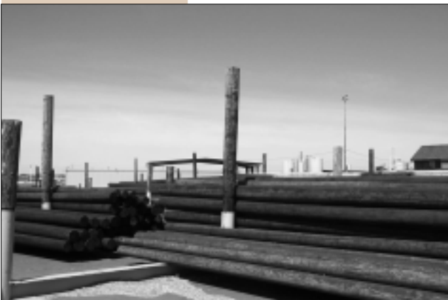
Four wood-treatment facilities in Washington use highly toxic pentachlorophenol to make wood utility poles resistant to rotting.
